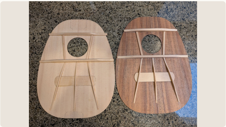
Completed top bracing: the destination for today's brace stock.
