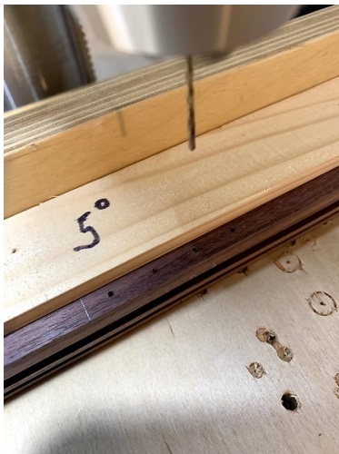
Drill holes at 5° angle
