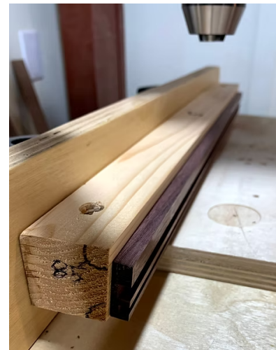
Scrap board with 5° "overhang" used on drill press.
