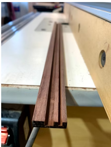
Routing the slots. If you have a long board you can make multiple bridges at once.
