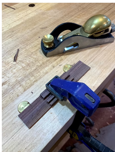
Using a block rabbet plane to clean up the wings.
