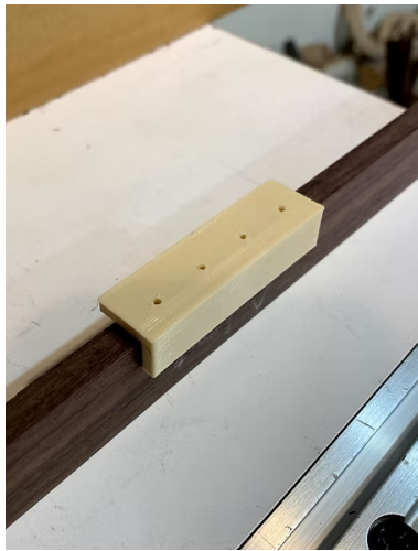
Simple 3D printed template for easy marking of hole locations.
