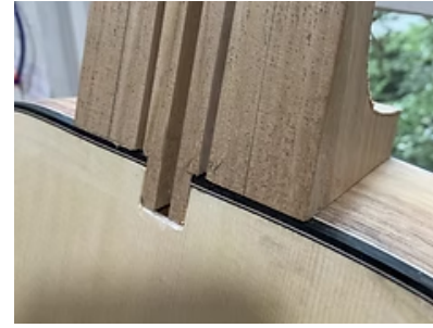
Rough fit of guitar neck to body.
