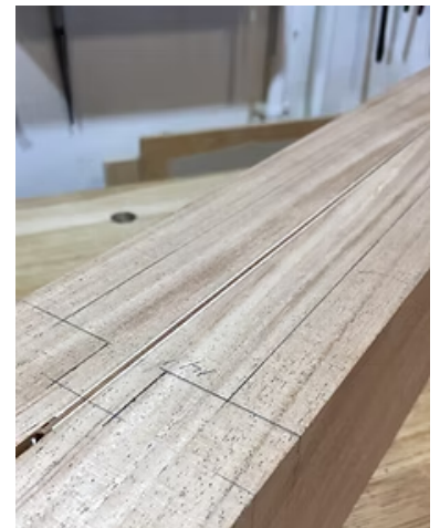
Laminated neck blank with layout.
