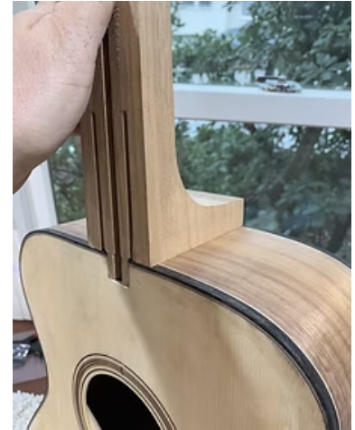
Final fitting of neck to guitar body. Neck and heel at final width
