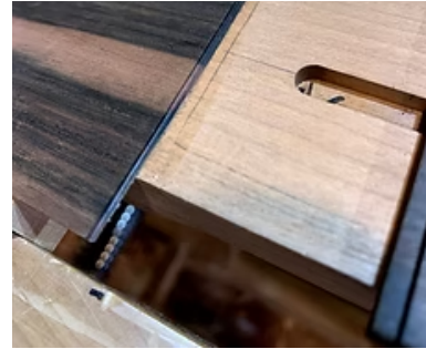
Nut (not shown) fits between edge of peghead overlay and end of fingerboard.
