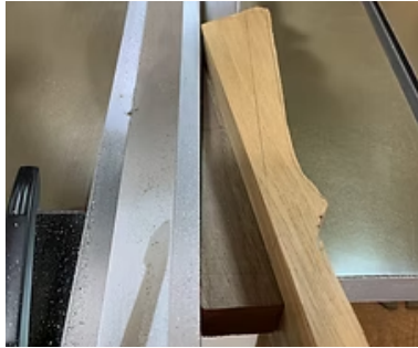
Cutting peghead angle with wedge in place.
