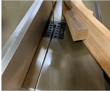
Taping wedge to neck to cut peghead angle on bandsaw.
