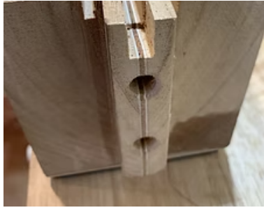
Guitar neck with slots for carbon fiber reinforcing bars and truss rod.
