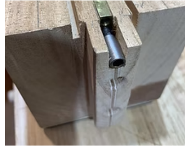
Guitar neck with truss rod.
