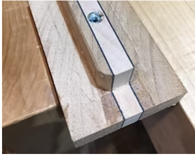
Ukulele neck with center slot for carbon fiber bar and bolt-on connection.
